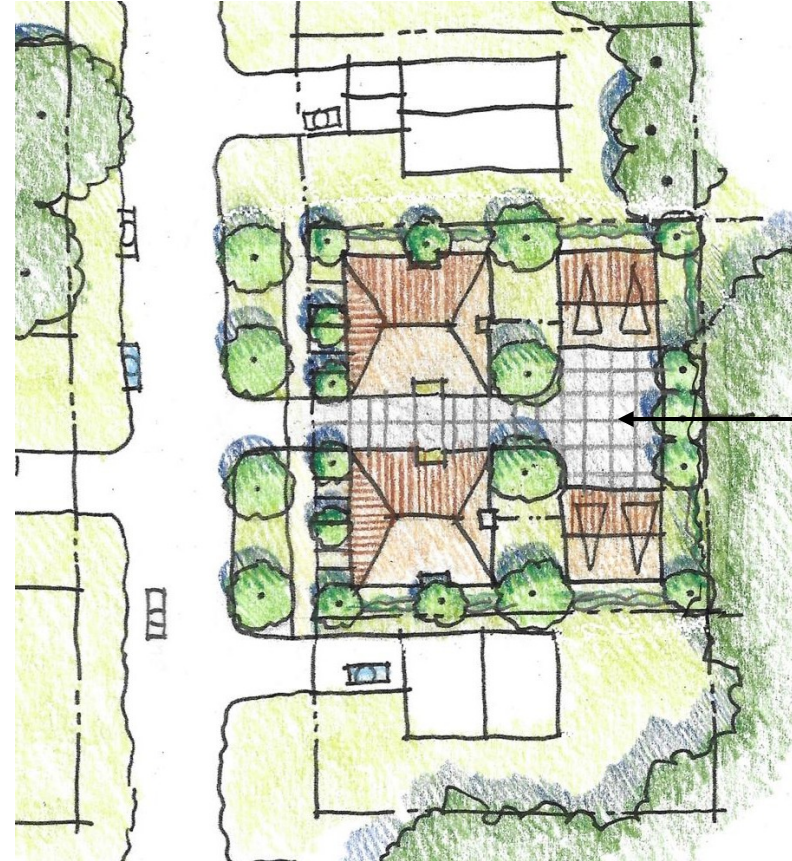
2 townhouse projects, with a shared driveway and two detached garages, no communal spaces
