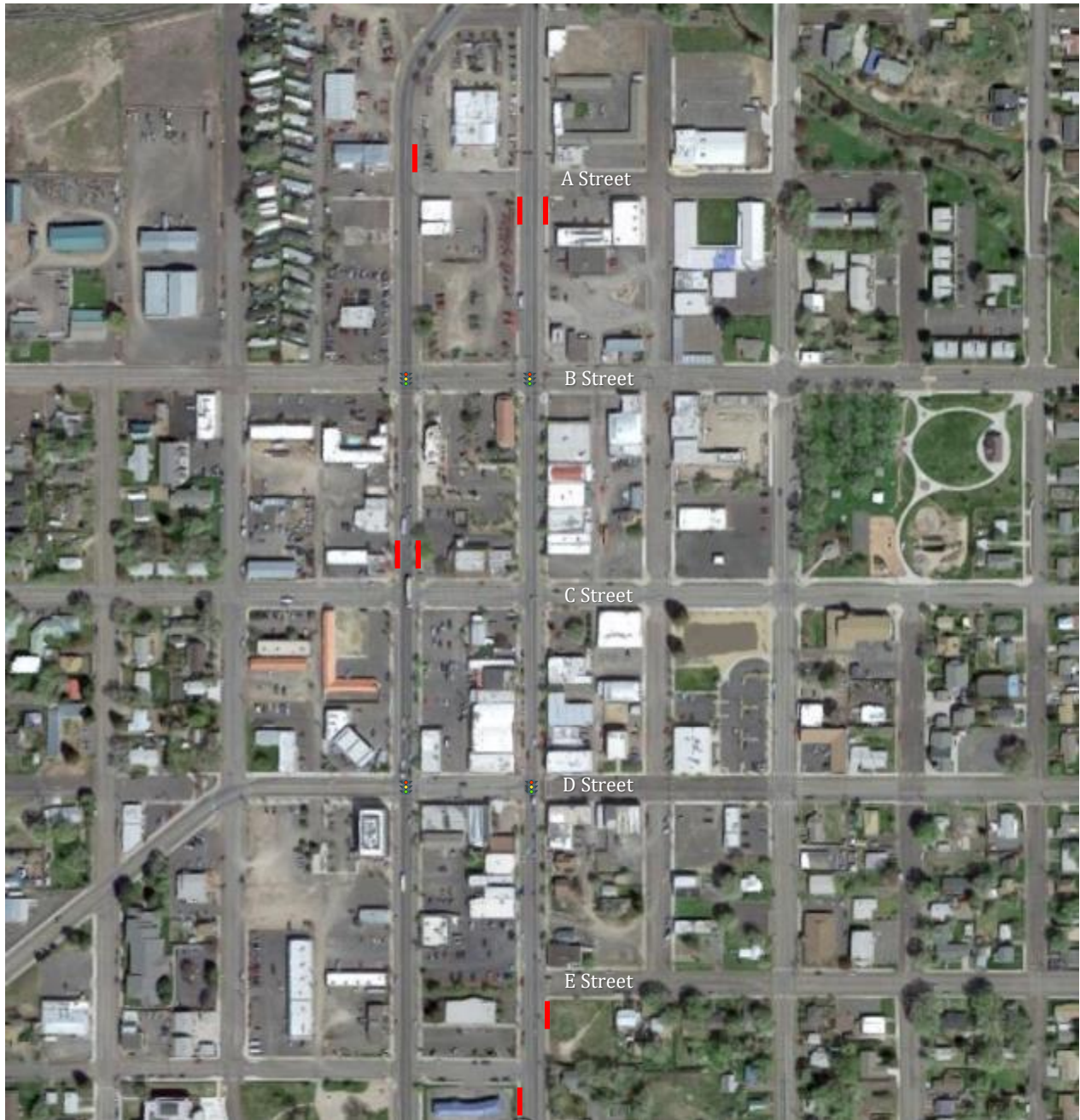
Figure L: Recommended sight line improvement locations (red stripes)
