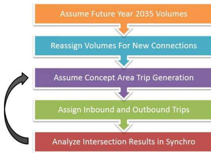
Figure 4: Analysis Procedures of Trip-Sensitivity Analysis
