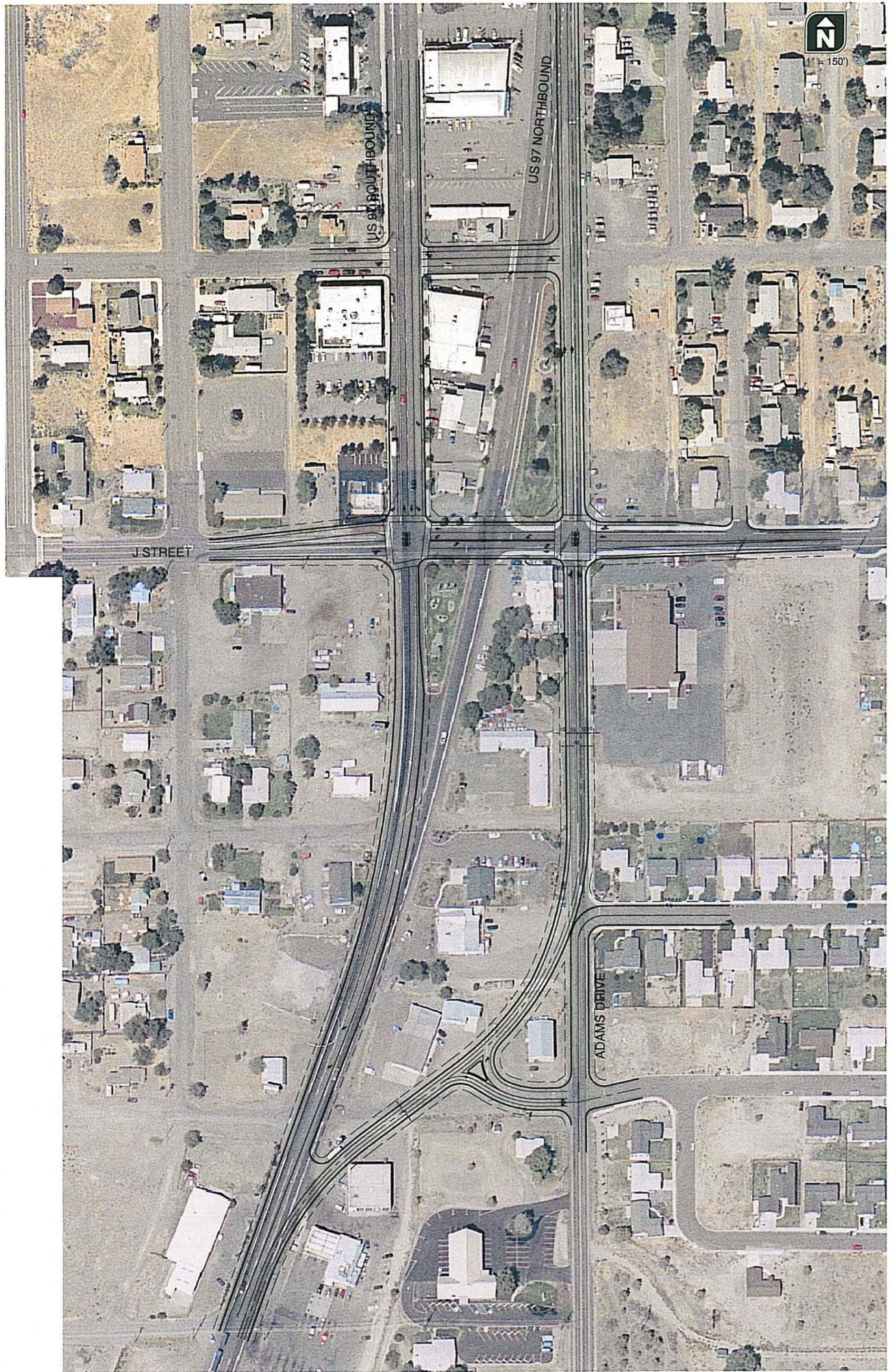
J STREET ALTERNATIVE SOLUTION C - DOUBLE-LINE DRAWING OF US 97/US 26 NORTHBOUND APPROACH REALIGNMENT MADRAS, OREGON
